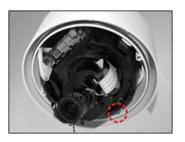
Step 8: Attach the Snap-on Camera Module to the Dome Camera Housing and tighten the Module-fastened Torx Screw.
