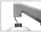
Step 2: Thread the Ethernet cable (and the power cable if applicable) through the entry of the Dome Camera's Housing.
