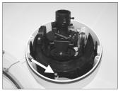
Step 6: Unscrew the module-fastened screw, as indicated in the picture.
