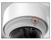
Step 11: Close the Dome Cover and tighten the Security Torx Screws. Replace the Dome Cover back, aligning the arrow mark on the Dome Cover with the one on the housing.
