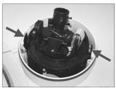
Step 7: Press the sides of the snap-on module, as indicated in the figure, and detach it from the Dome Camera's housing.
