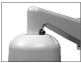
Step 3: Rotate the joint of the Dome Camera Housing into the entry of the Wall Bracket, aligning the screw hole of the joint with the one of the Wall Bracket. Fix the camera housing with the supplied M8x12 Screw and Washers.
