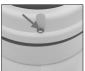
Step 4: Use a Security Torx to unscrew the two Torx screws on the side of the Dome Cover, as shown in the figure, and open the Dome Cover. The Security Torx is included in the package of the camera.
