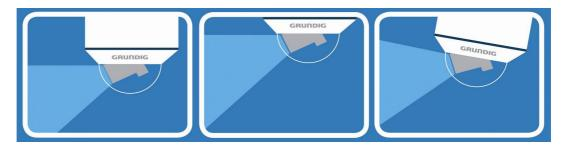
With standard bracket, Vandalproof dome allows only tangential view along the lid. The bracket enables inclined by increasing the angle of vision to monitor the wall supporting the camera. It is ideal for monitoring of ATMs, access, display cases.
