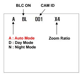
Note) Icon or abbreviation of the function will be displayed for about 5sec When corresponding key is pressed
