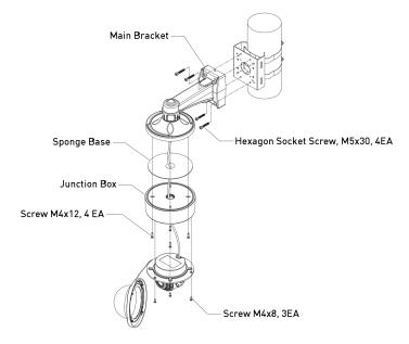
Furthermore, it is possible to use the GBR-FB03 and to mount a matching Integrated Camera/Bullet Camera on it.
