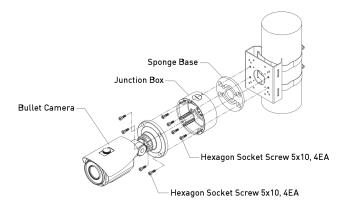
Make sure the cables are led freely through the Bracket as shown in the previous drawing and that all screws are fixed tightly.
