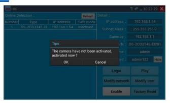
1. Hikvision activation: When connect the unactivated Hikvison camera to the tester, it will auto identify and display "Unactivate" at safety mode. Select needed activate the camera, click bottom right corner button "Enable", pop-up "the camera is not activate, activate now"?
