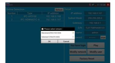
If the camera not supports non-verification login, pls select "camera" of online detection menu, and input correct user name and password, then click "log in". After logging successful, you can test it.
