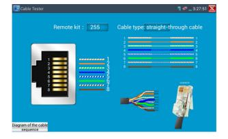
Test LAN cable or telephone cable.
