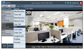
**Zoom in image**: press the key to enter the zoom mode. Press it again to exit zoom mode. When the image is enlarged tap left, right, up or down on the image to move the whole image on the screen
