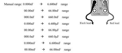
d. Before connect test leads across two sides of the capacitor under measurement, be sure that the capacitor has been discharged fully.
