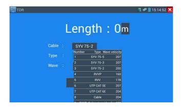
User-defined calibration: Choose the cable 100 meters to 200 meters (more than 50 meters), click "Cable", "Type" to select user-defined 1 for calibration, 11 groups user-defined can be set.
