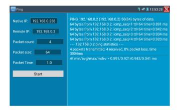
**Application:** PING testing is the most conventional network debugging tools. It is used for testing if the connected IP camera or other network equipment's Ethernet port is working normally and the IP address is correct.
