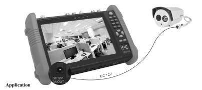
Power output function is mainly used in the camera field demonstration and testing, meanwhile, for some camera installation sites, If there is no power outlet for the adapter to power the camera, the tester can offer temporary power for it. But we do not suggest tester supply power for a long time.
