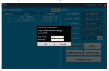
Factory reset setting: camera will be soft reset, and the device's user name, password and network set
