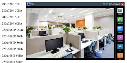
When SDI tester detects the camera input image resolution is 1080p 60Hz or1080p 50Hz, the tester's screen will display "Does not support playing 1920\*1080p 60Hz".
