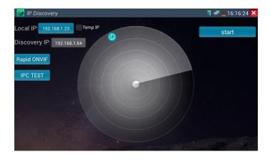
**Local IP:** Tester's IP address, Tester can auto-modify the tester's IP to the same network segment with the scanned camera's IP
