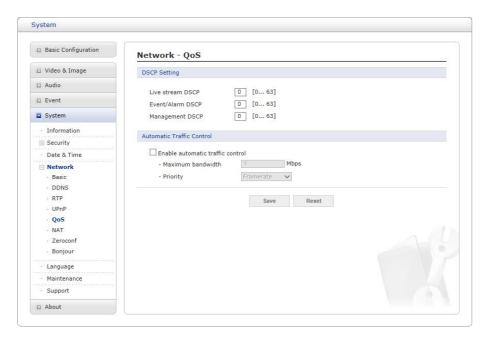
Quality of Service (QoS) provides the means to guarantee a certain level of a specified re-source to selected traffic on a network. Quality can be defined as a maintained level of bandwidth, low latency, and no packet losses.
