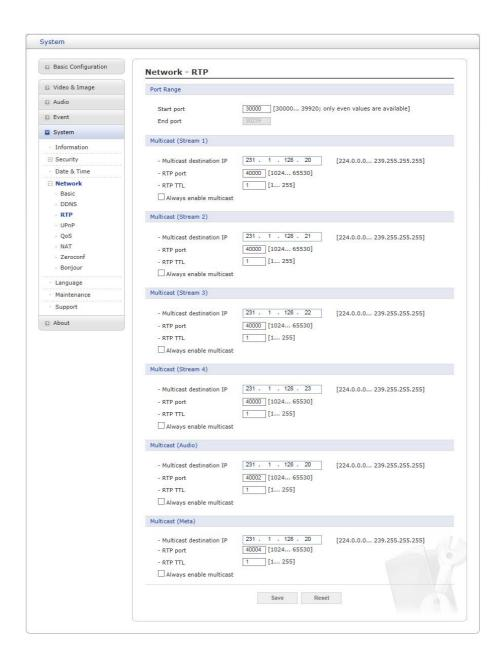
Create a setting for sending and receiving an audio or video on a real-time basis. These settings are the IP address, port number, and Time-To-Live value (TTL) to use for the media stream(s) in multicast H.264 format. Only certain IP addresses and port numbers should be used for multicast streams.
