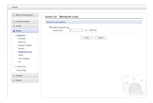
This is used to trigger an event every time the network connection is failed.
