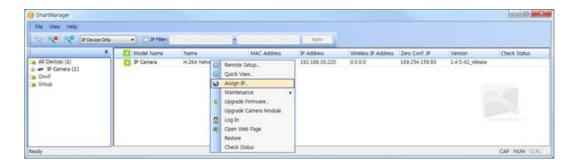
4) Select Assign IP Address. The Assign IP window will display. Enter the required IP address.
