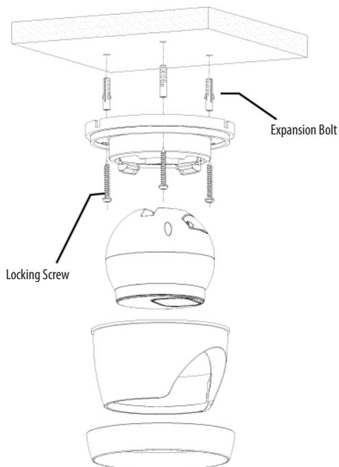
Fix the pedestal by drilling locking holes around the sticker and inserting three expansion bolts into the holes and fastening it with three locking screws.
