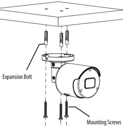
Insert three expansion bolts in place into the ceiling and fix the equipment with three mounting screws.
