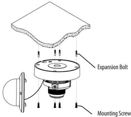
Use the position indicated on the position sticker to drill the holes needed to mount the camera base. Insert the expansion bolt into the holes. Match the base's mount openings to the expansion bolts position, then place the mounting screws through the base's mount opening into the expansion bolt. Tighten the mounting screws to ensure the camera base mounted securely.
