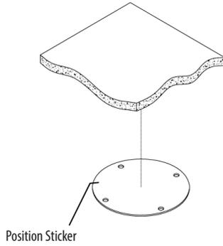
Apply the position sticker to the desired camera mounting position.
