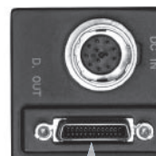
Small SDR (Mini-CameraLink) Connector [24.4 x 9.0 mm]
