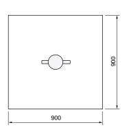
Set bollard into foundation. Fill bard with concrete - capping plate has rags on underside to push into the concrete filled bollard holding plate in position once concrete has set.
