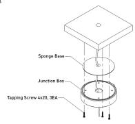
Make sure the cables are freely led through the Junction Box as shown in the drawing and that all screws are fixed tightly.
