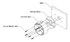
Make sure the cables are freely led through the Junction Box as shown in the drawing and that all screws are fixed tightly.
