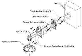
Make sure the cables are led freely through the Bracket as shown in the previous drawing and that all screws are fixed tightly. Connect the Dome Camera to the Wall Bracket as shown in the following drawing.
